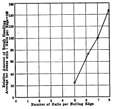
Fig. 50.—Tests on nailed boxes for two dozen No. 3 cans; relation of number of nails to amount of rough handling required to cause loss of contents.
